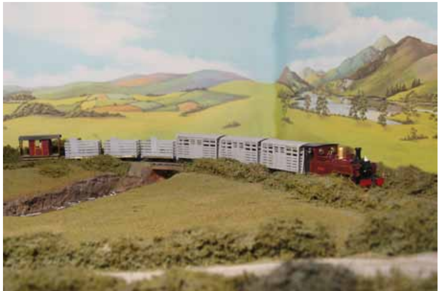
Russell hauls the new Llanmynach & Tawel-Llety Railway livestock train over the Nant Fernol bridge on the first trial run, unpainted and part complete! The vehicles are mounted on Peco N Gauge underframes to ensure they remain compatible with the existing rolling stock which is nearly 30 years old. The solebars are 3/32" square solid brass bar to give a little weight and improve the wheel/rail interface. Photo: David Burleigh .
